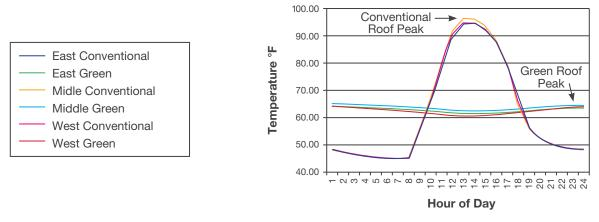
The daily range in temperatures for the exposed and Green Roof is 600°F and 60°F respectively. Large ranges in maximum and minimum temperatures over the 24 hour cycle causes severe heat stress on all the roof components including expansion and contraction and out gassing of volatiles. This also means the surface waterproof covering is more likely to fail early.
